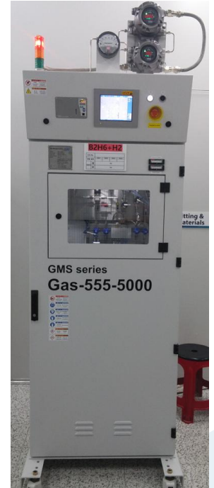
Gas mixing system Concentration control Application: B2H6
