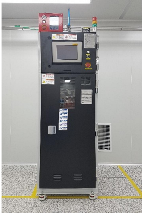
N2 Purge Concept (DTLR) Application: TEOS, TiCl4, BDEAS, HCDS...
