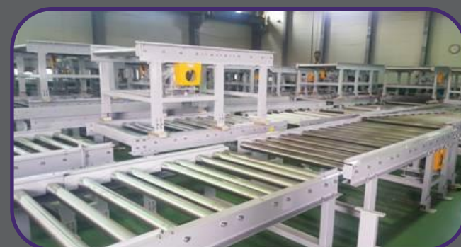
Logistics Transfer Roller Conveyor (1)
