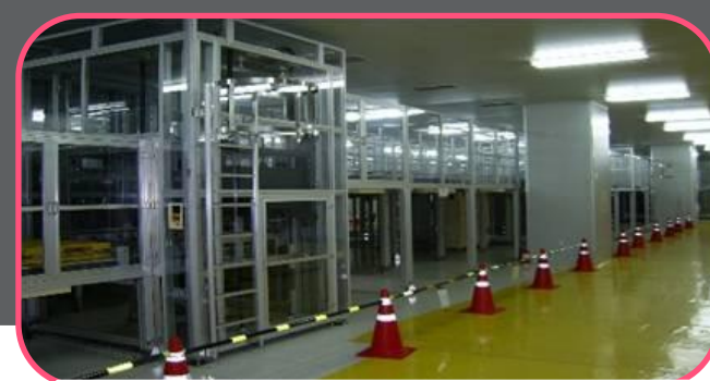
Pallet Transfer Lifter & C/V
