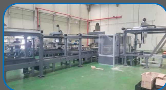
Pallet Transfer Line
